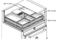
Residual temperatures of the heating rack in the top cabinet approximately 150°C, based on the oven working at 300°C.
